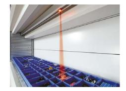
**Position Indicator Light Bar:** Incorporated into the access openings of both vertical lift modules and vertical carousels, these LED lights illuminate in alignment with the position of the required item where it is stored in the tray.
