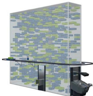
**Vertical Buffer Modules (VBM)** –In the middle of a multi-segment shelving system is an aisle, where a moveable mast with a telescopic gripper operates. The control unit sets the gripper in motion picking a bin and transporting it to a picking station.
