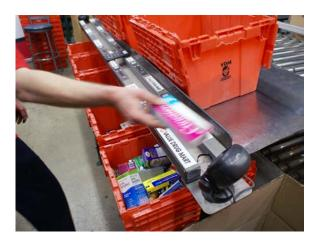
To reduce labor requirements and speed picking productivity, Value Drug Mart in Edmonton, Alberta (Canada) replaced two zones of static shelving with six horizontal carousels integrated with pick-to-light technology. Stacked and organized into two zones of three carousels each, picked items are batched into orders, with a batching station that accommodates simultaneous fulfillment of up to 10 orders.
