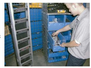
**Put/Batch Lights:** Used with both horizontal and vertical carousels, as well as VLMs, these light-directed picking modules direct an operator to put or store items in a specific or active location when replenishing stock. They can also be used for order consolidation, batch picking and sortation at workstations located near the automated storage and retrieval units.
