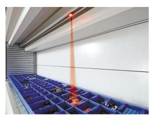
**Position Indicator Light Bar:** Incorporated into the access openings of both vertical lift modules and vertical carousels, these LED lights illuminate in alignment with the position of the required item where it is stored in the tray.
