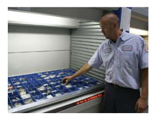
Light Pointer: Used with VLMs, this system deploys an LED or laser light mounted on a slider that moves horizontally on a guiding system within the access opening of the storage and retrieval unit. Software-driven, the light pointer also swivels to project the light beam in the depth direction of the machine to illuminate any position within the storage tray. The light spot identifies the precise location of the item to be picked or replenished, eliminating search time.
