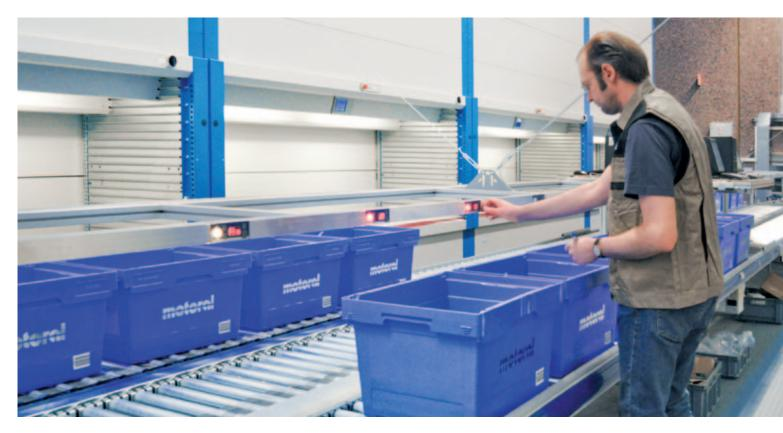
The amount of order picking locations and pick-to-light displays and the buffer capacity are determined by customer specific demands.
